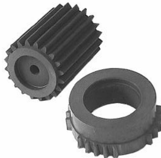
Copper and graphite electrodes with toothed profiles
