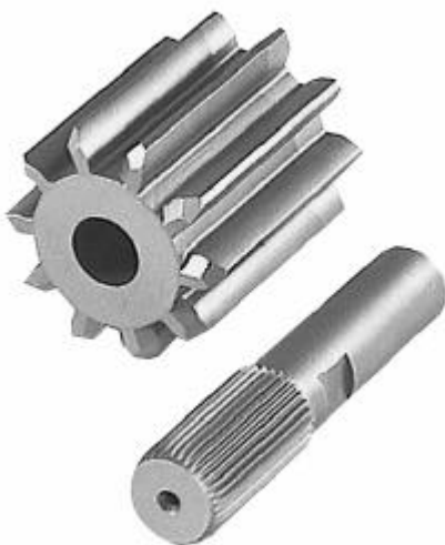
Copper and graphite electrodes with toothed profiles
