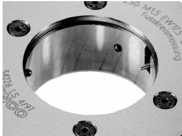
Hand held indicating ring gage for minor diameter
