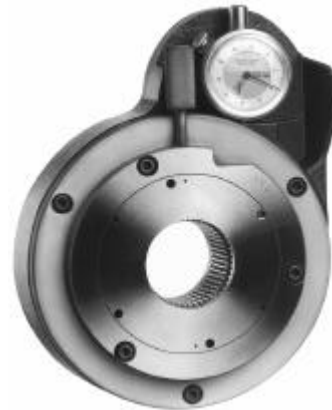
Hand held indicating ring gage for external splines
