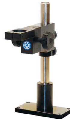
MA 331 / MA 333 / MA 335 / MA 336 - Displacement with geared drive, range 40 mm - Normal displacement or normal and fine displacement - Column length 300 mm, quick displacement 130 mm - Column length 400 mm, quick displacement 230 mm - Column length 500 mm, quick displacement 330 mm For all bases
