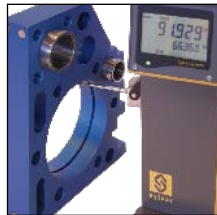
Internal measurements with ruby ball probe Ø 3 mm, 930.2101 (standard)
