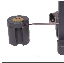
Taking the probe constant value with the setting bloc 930.2002 (standard)
