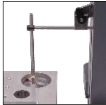
Internal groove measurements with accessories 930.2108, 930.2110 and 905.2207
